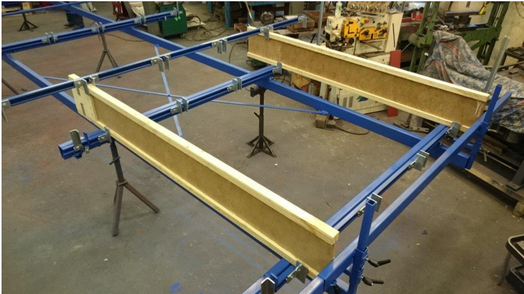
Jigg for gulv/tak elementer
